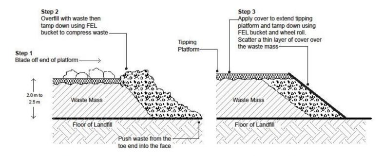
Note — Tamp down the exposed waste with the FEL bucket from the top and then, if accessible, from the toe area push any loose waste into the leading face. Then tamp in the exposed waste with the FEL bucket. Scatter some soil over the leading face from the top (and from the bottom, if accessible) after tamping is completed. This will save cover material and reduce windblown litter
