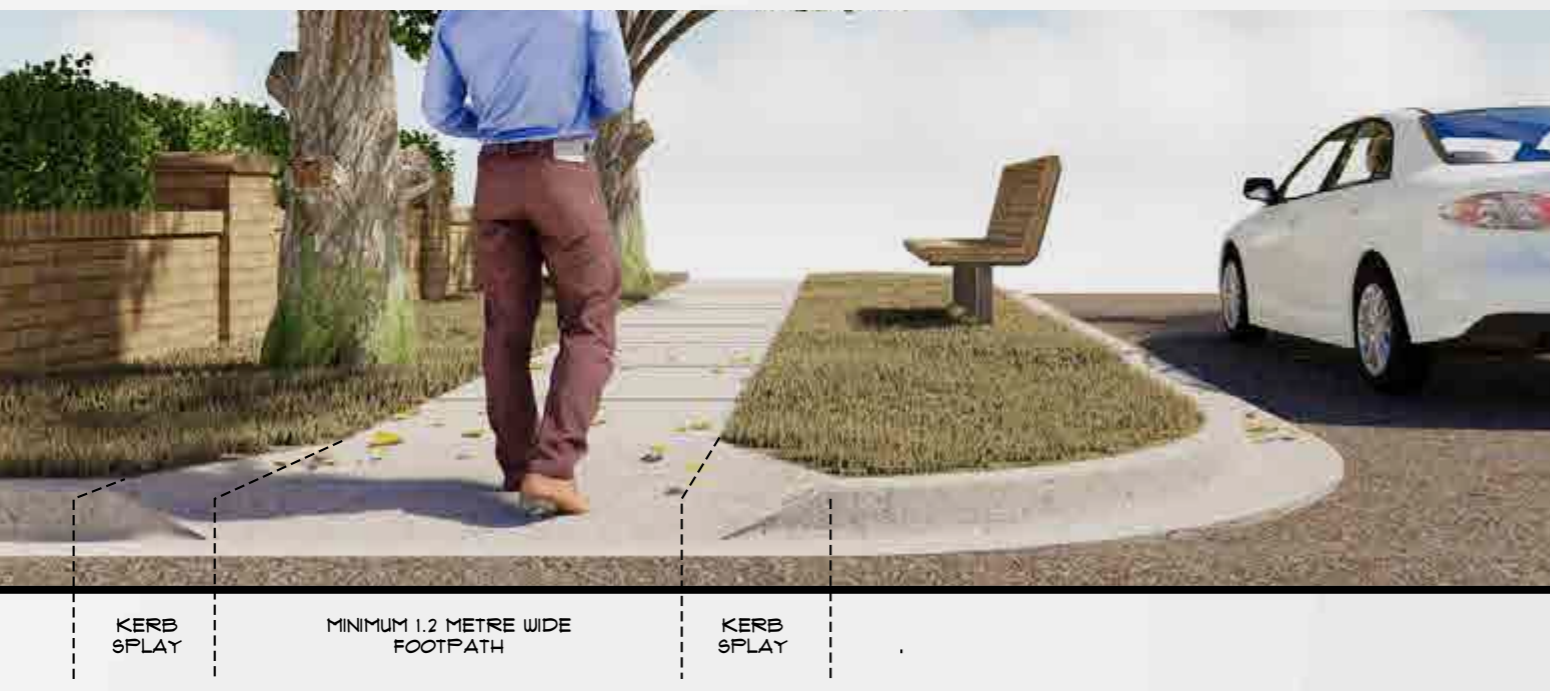
Typical Compliant Kerb Ramp Arrangement
